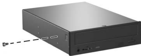
Figure 7-23 Installing the Guide Screw in the Optical Drive
